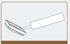
Installation Tips: Apply silicone inside of cap. Do not apply to post and then slide cap on. Do not add silicone to any other parts that it is not intended for.
