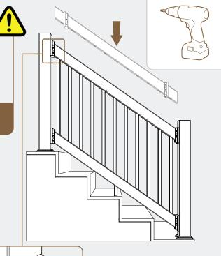
**Installation Tip:** prior to cutting, use a soft clamp to lock the bottom rail in place against the post and then mark the cut lines.
