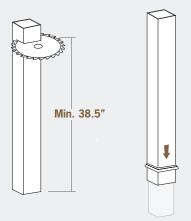
Min height of the post at the top of the stair section is 38.5". The post at the bottom of the stair section should be taller than 42".
