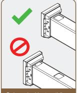
End cap should not partially cover over a baluster cut out.
