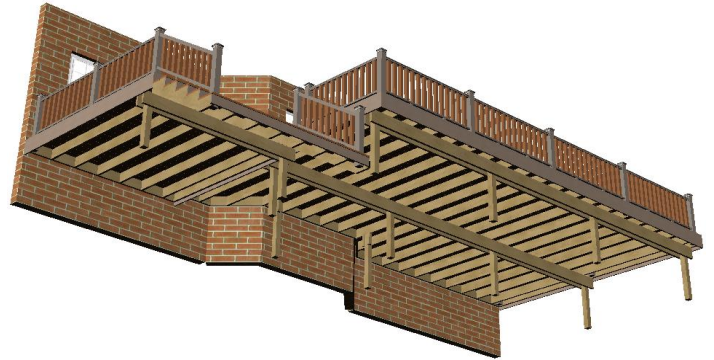
Bottom view with planks
