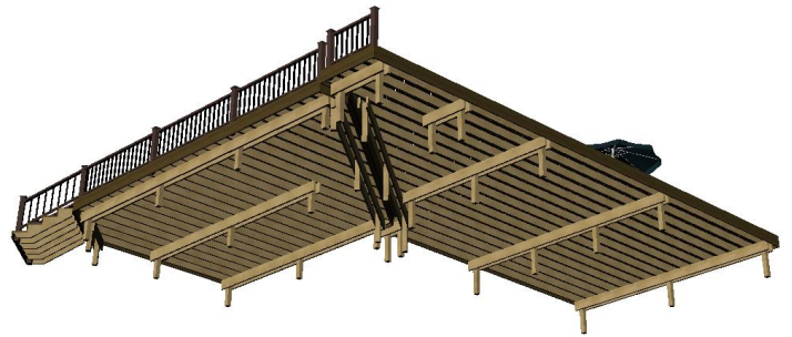
Bottom view with planks
