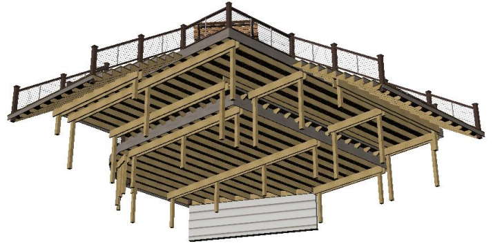
Bottom view with planks
