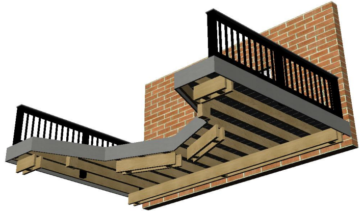
Bottom view with planks
